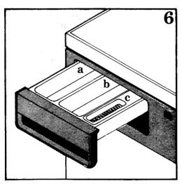
Pull out the dispenser and add the measured amount of powder, following the directions on the wash powder packet (see also Table below). Be sure to use enough powder — this is essential to get the clothes really clean. Once the dispenser is filled, close it by pushing it in gently. This is particularly important if you are using a fabric conditioner because if the drawer is slammed it will cause the conditioner to enter the machine prematurely.
